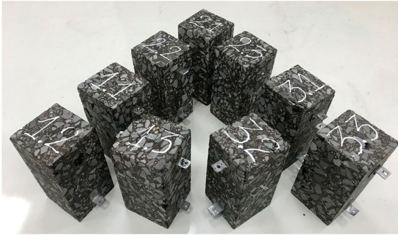
Figure 1. Preparation of samples for AC, PMB, and HiMA mixtures.
